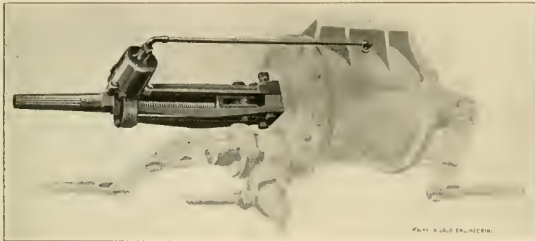
FIG. 1. ATTACHMENT OF SLACK ADJUSTER TO BRAKE CYLINDER.
